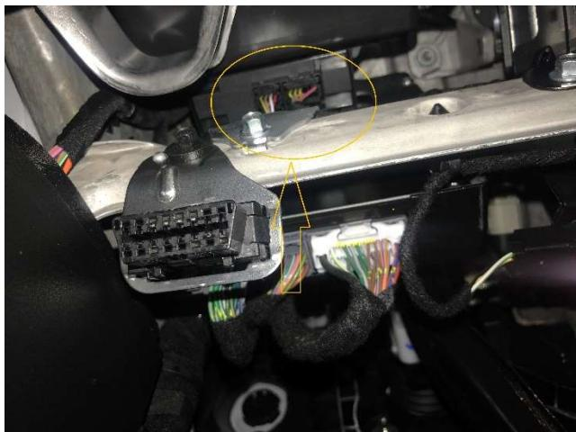
into the Tazer JL lite. The Tazer JL Lite typically should be left installed unless the Jeep is going for dealer service. It does not need to be plugged in for any of the features in the *Vehicle Settings* to remain operational.
